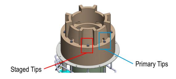
Figure 12 Advanced burner tile design to help minimize NOx formation.
