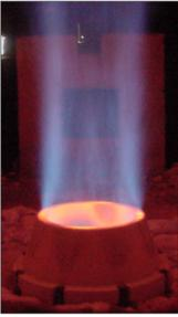
Figure 9 Burner with a round tile.
