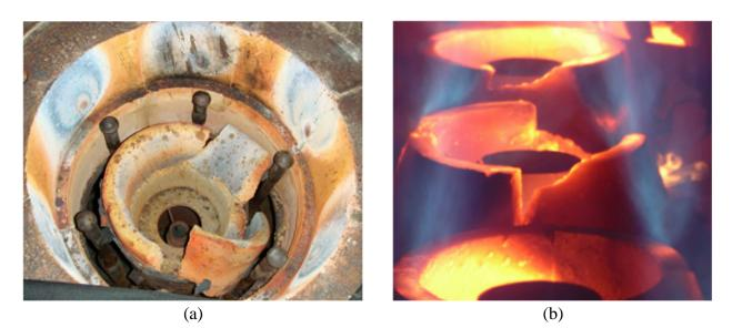
Figure 18 Damaged (a) regen tile, (b) burner tiles.
