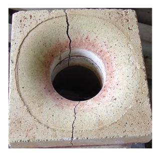
Figure 17 Cracked burner tile.
