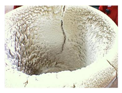
Figure 20 Catalyst build-up on a regen tile.
