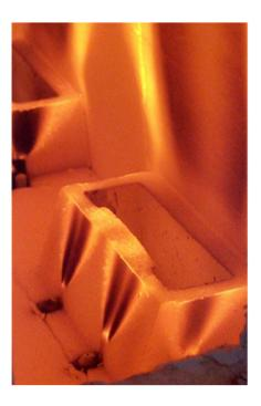
Figure 10 Burner with a rectangular tile.
