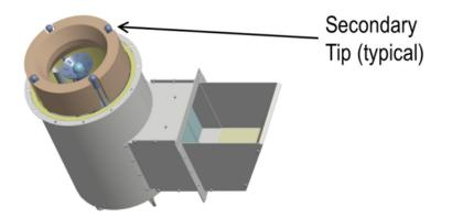
Figure 11 Burner tile with secondary fuel tips in the tile.
