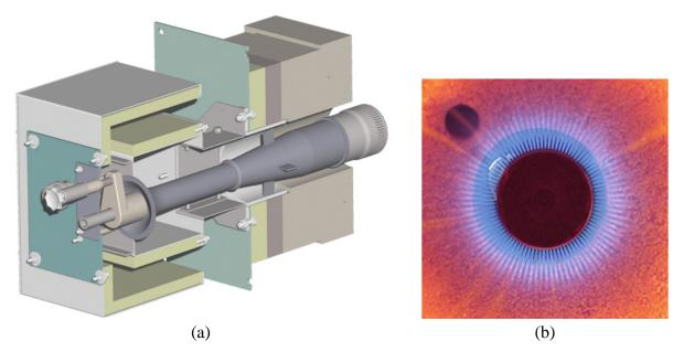
Figure 1 Radiant wall burner: (a) cutaway, (b) photo of burner radiating in a furnace.
